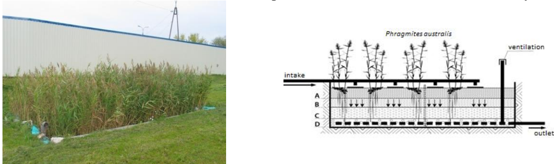
Fig. 1. Installation 3 and VFCW cross section scheme [2]
